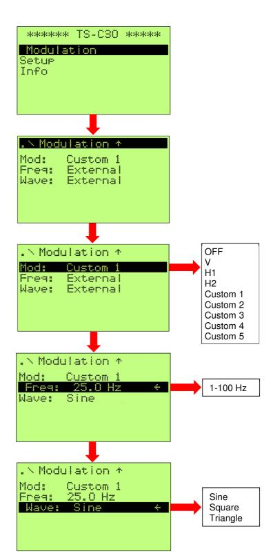
To view those functions turn the "MOD.LEVEL" knob clockwise to enable the internal signal generator!
